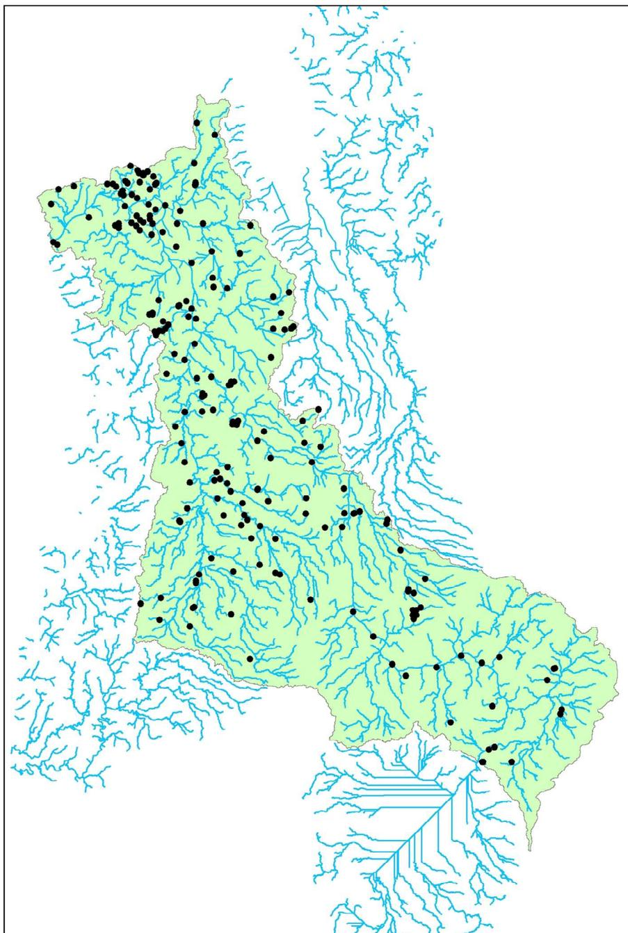
**Figure 1:** Location of dams listed in the NIWA database within the Waikato River catchment area (shaded in green) overlain on the River Environment Classification (REC) stream network showing third to seventh order streams.
