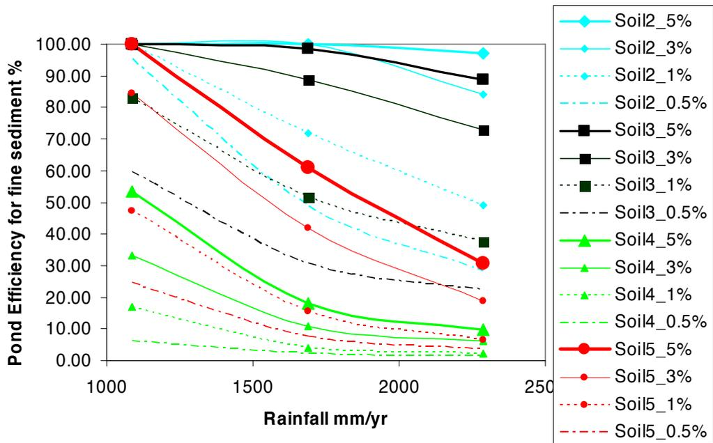
**Figure 2:** Simulation results for pond performance for fine sediment removal as a function of pond size (percentage of catchment area drained) and catchment soils. Soil 2=very well drained; 3 = well drained; 4 = poorly drained; 5 = average drainage.
