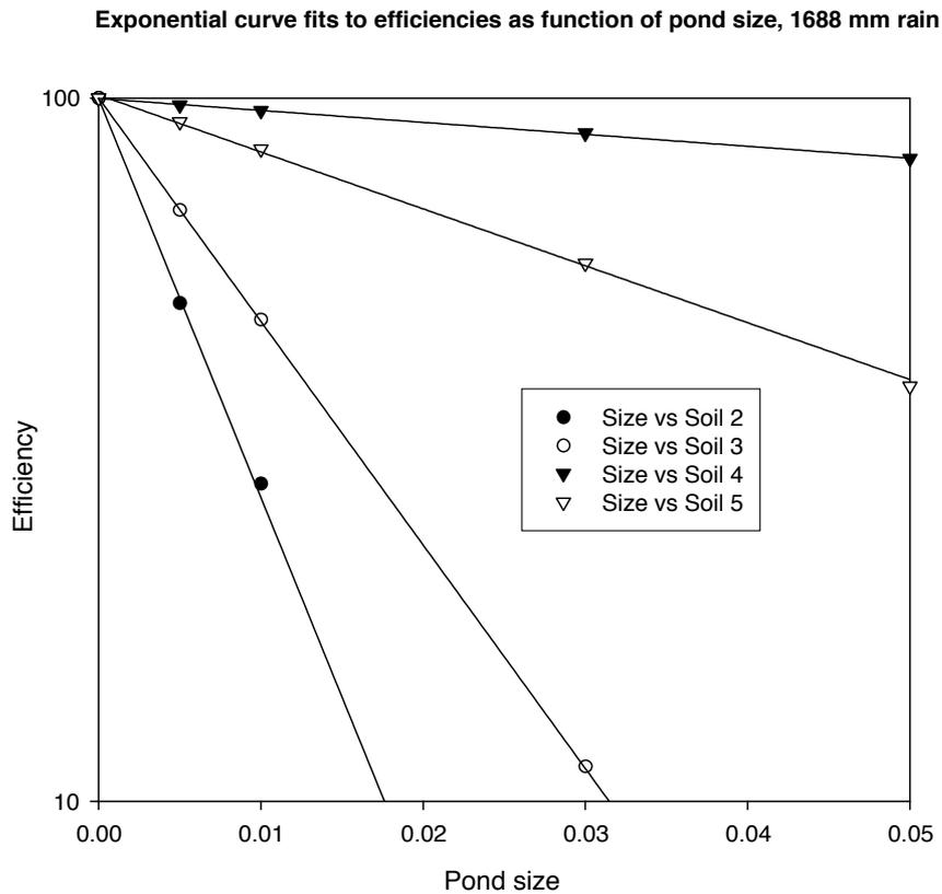
**Figure 3:** Fine sediment removal efficiency curves for a typical Waikato hill rainfall in relation to pond size and soil type.
